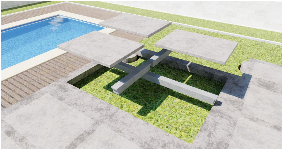
Figure 4 - Floor joists and panels stacked on top of foundation pier pads
